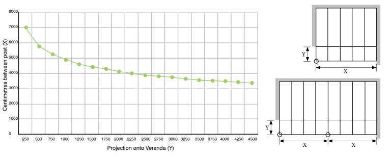
For loading condition other than 0.6kn/m2 (with 4-16-4 glass units) please let our specification team know. Ultraframe's U-Design software simply needs your home postcode to calculate the loads and the resulting roof specification.
